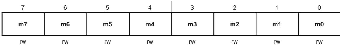
**UxMCTLx**      Bits              The modulation control register is not used for SPI mode and should be set to 000h.
