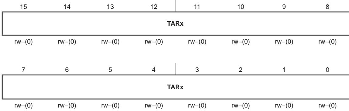
**TARx**      Bits      Timer\_A register. The TAR register is the count of Timer\_A.
