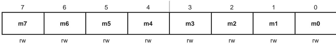
**UxMCTLx**      Bits      Modulation bits. These bits select the modulation for BRCLK.
