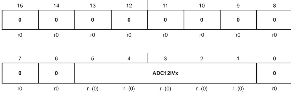
**ADC12IVx**    Bits    ADC12 interrupt vector value
